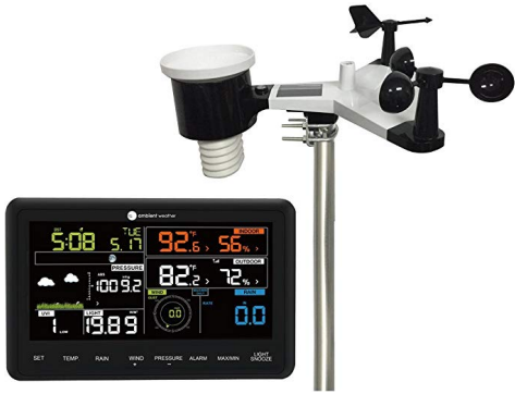
Fig. 4. The Ambient Weather WS-1900 Osprey weather station [7]. This system sends sensor data to api.ambientweather.net but it can be converted to send data to a user-controlled Wattsworth node instead. This removes the dependence on a third party for data collection and storage.
